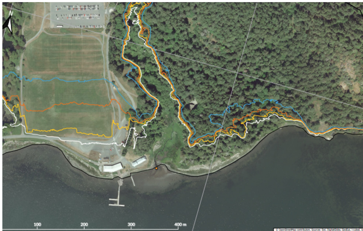
Coastal flooding and inundation mapping showing scenarios on the Royal Roads University lands. Source: Associated Engineering & DHI Water & Environment Inc. mapping for City of Colwood.
