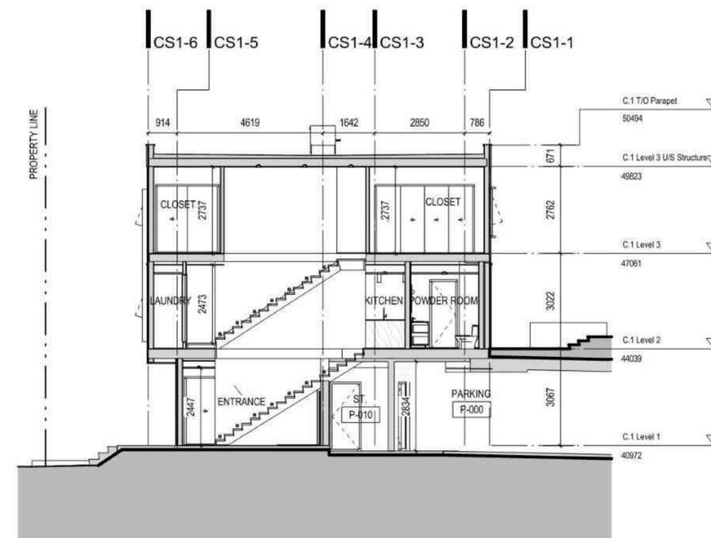
3 Building Section - C.1 NS Stairs 1:100
