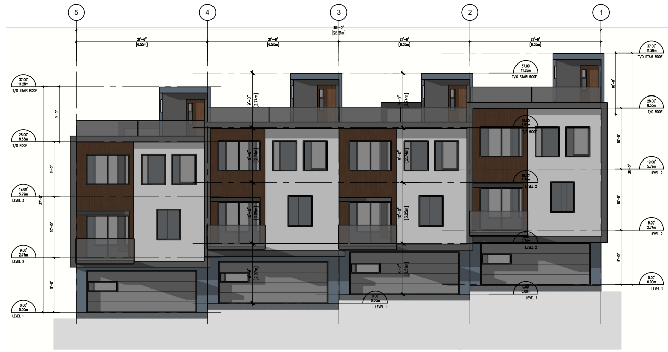
2 BLOCK 1 - NORTH ELEVATION A1-301 1/16" = 1'-0"
