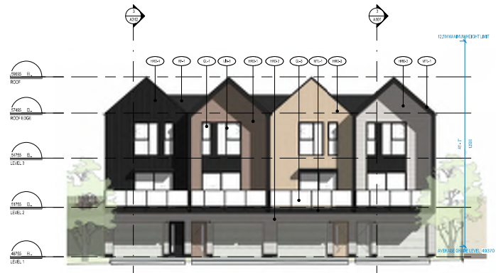
3 BLOCK E - EAST ELEVATION 1:100
