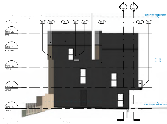
1 BLOCK H - EAST ELEVATION 1:100
