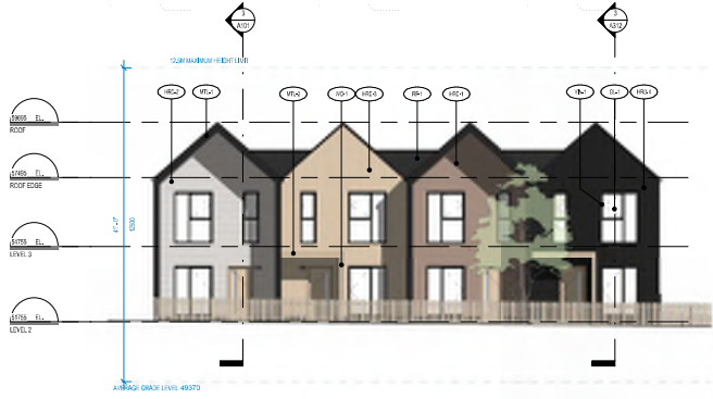
1 BLOCK E - WEST ELEVATION 1:100
