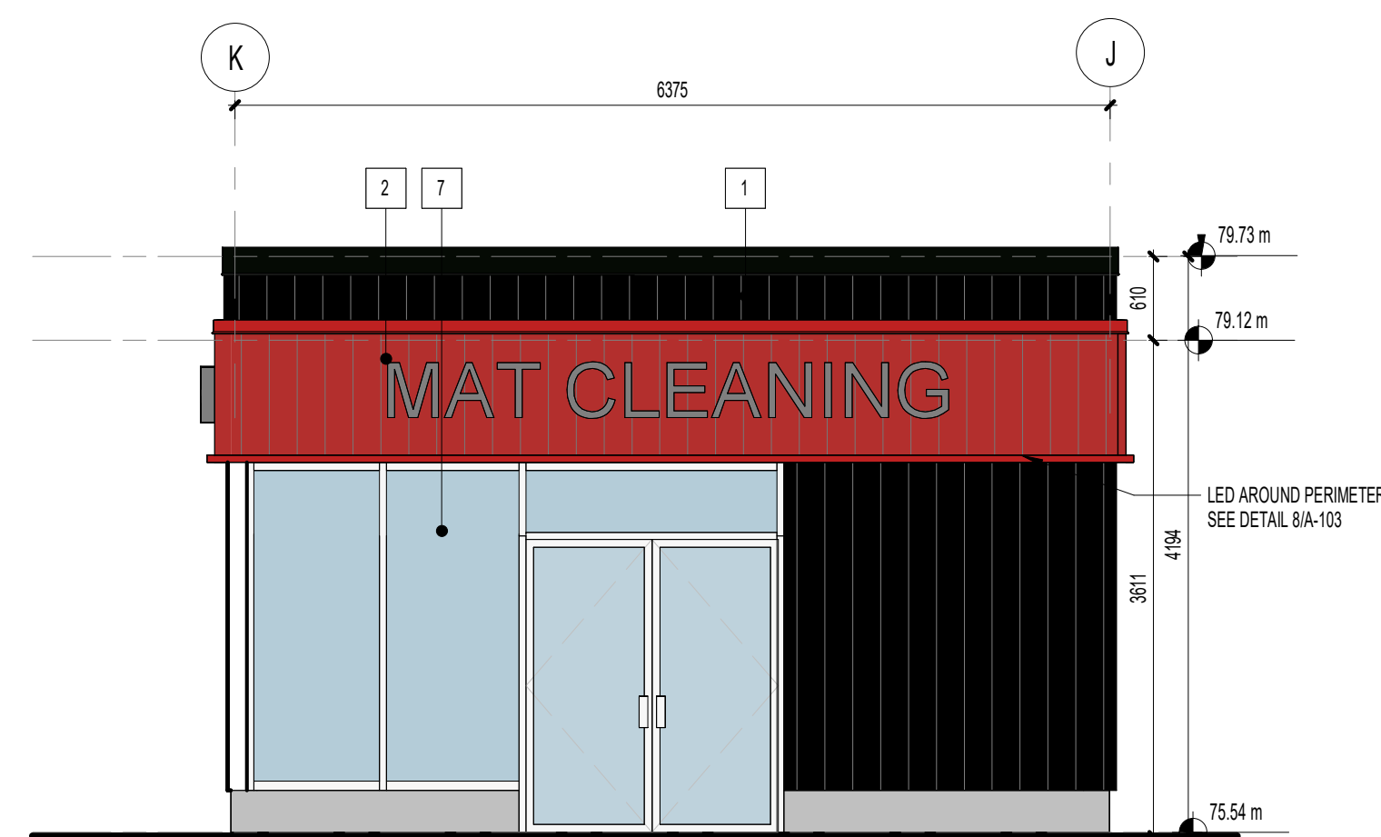
4 SOUTH ELEVATION- MAT CLEANING A-103 SCALE: 1 : 50
