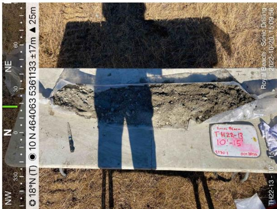
Photo 4. Example of Colwood sands and gravels encountered at TH22-13, depth 3.0 m to 4.6 m bgs.
