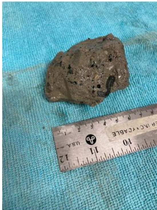
Photo 6. Chunk of intact till-like soil from 16.3 m depth at TH22-13 following soaking.
